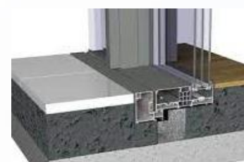
Slim Sliding- Imbedded- 3D Detail
