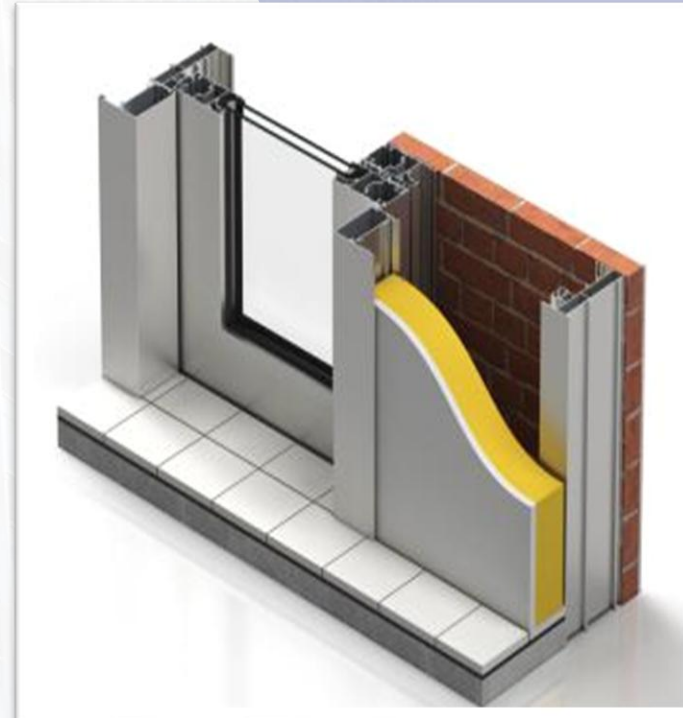
Sliding door hidden the wall- 3D Detail
